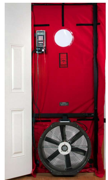
Blower door installed and ready for testing.
