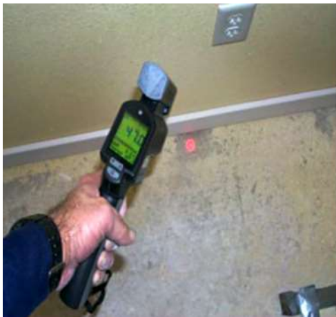
Air leakage at the exterior wall floor junction.
